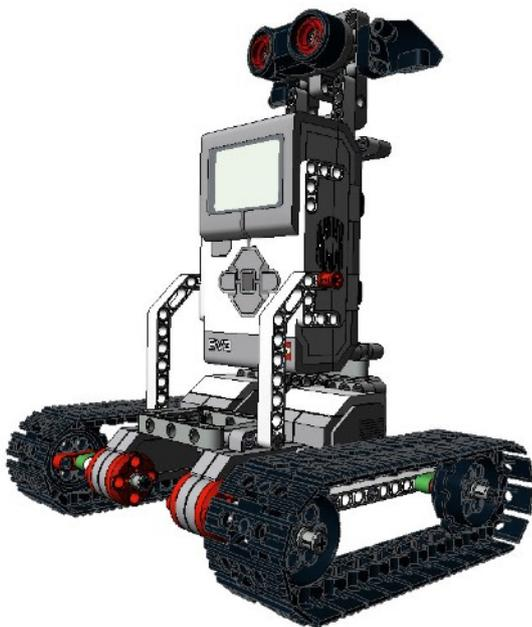
Tank Bot is an all-terrain autonomous robot. Tank Bot uses the Random Function to decide on where it will go next. The display screen displays eyes that determine Tank Bot’s direction of travel. The Tank Bot Ultrasonic Navigator uses the ultrasonic sensor to detect the proximity of obstructions. When it gets too close to something, the program uses a random block and a switch to decide which way to turn away from the obstacle.
